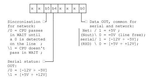
OBS: Because the ports (#F7) and (#EF) are decoded incompletly, when selected with (A3=0), and (A4=0), they may be selected simultaneoulsly, improving the way that the bits are arranged in the bus:
